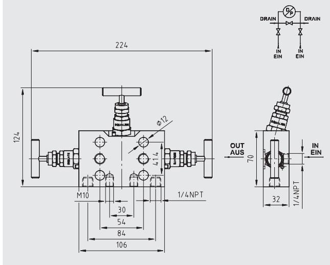
With upstream pressure equalising valves it is possible to avoid unilateral overpressure loadings during both start-up and operation as well as enabling zero point checks during operation. Furthermore, they enable the isolation of the process lines without interference to the running process.
