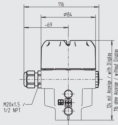
Single chamber housing, cast stainless steel
