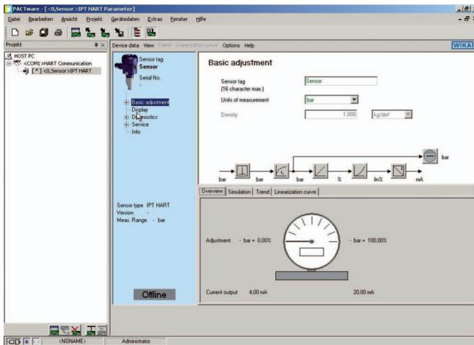
For HART output signals, Profibus-PA and FF, a DTM is available in accordance with the FDT-standard. The DTM provides a self-explanatory and clear user interface for all setup and control processes of the transmitter. For testing purposes, it is also possible to simulate process values and archive the parameter data. Recording of the measured values is available for diagnostic purposes.
