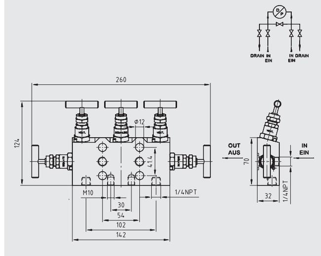
These pressure equalising valves with integrated shut-off valves, and also purge and ventilating valves, in addition enable the venting of the pressure gauge on one or both sides and enable the supply line to be purged.
