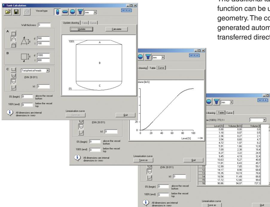
The additional tank volume calculation of the DTM function can be used to reproduce any optional tank geometry. The corresponding linearisation table is generated automatically. The linearisation table can be transferred directly to the transmitter.
